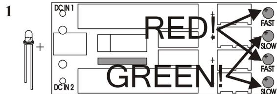
Begin by inserting the 8-pin resistor pack and the four light emitting diodes (LEDs). The resistor pack can be inserted in either orientation, but the LEDs are polarized. Make sure to put the longer, positive leads into the holes marked with '+' on the PCB silkscreen. Use the red LEDs for the 'FAST' indicators and green LEDs for the 'SLOW' indicators.
