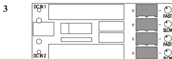
Now, add the four battery connectors. Pay attention to the polarity-indicating tabs on the connectors, and align them with the marks on the PCB silkscreen. In general, make sure the positive terminal of the battery you are charging is on the side marked '+'.
