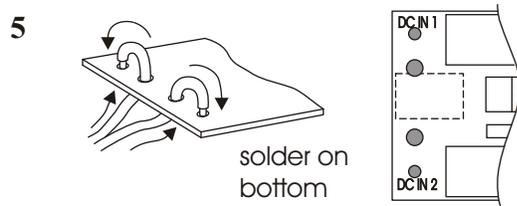
Finally, connect the power supply leads to the PCB. Pass the insulated wires through the larger, inner holes from the bottom of the board, then bend them out and solder them to the outer holes. The larger holes and the wire insulation provide a strain relief that should prevent your wires from breaking off with use. Either wire can go to either hole. J1, a DC input jack, is not used this year.
